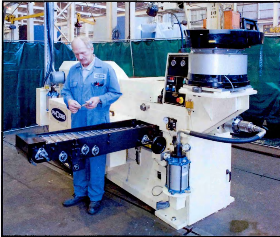
Figure 53: View 2 - Typical Joseph Rhodes Knuckle Joint Press
