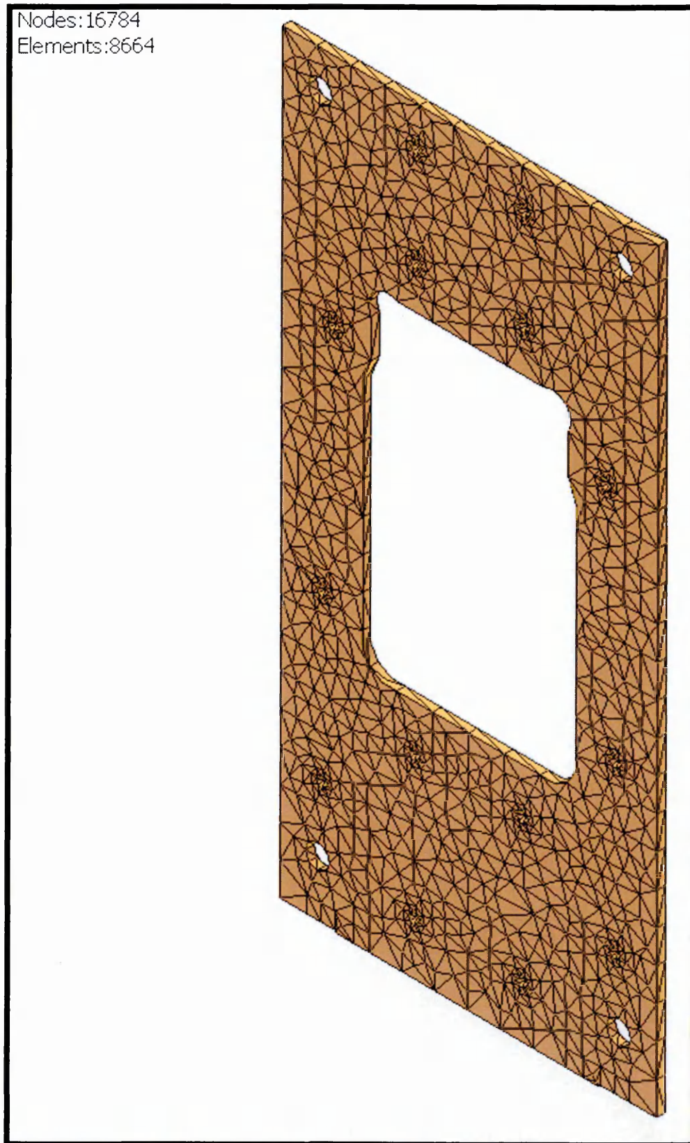
Figure 31: Frame plate - Geometry and Mesh
