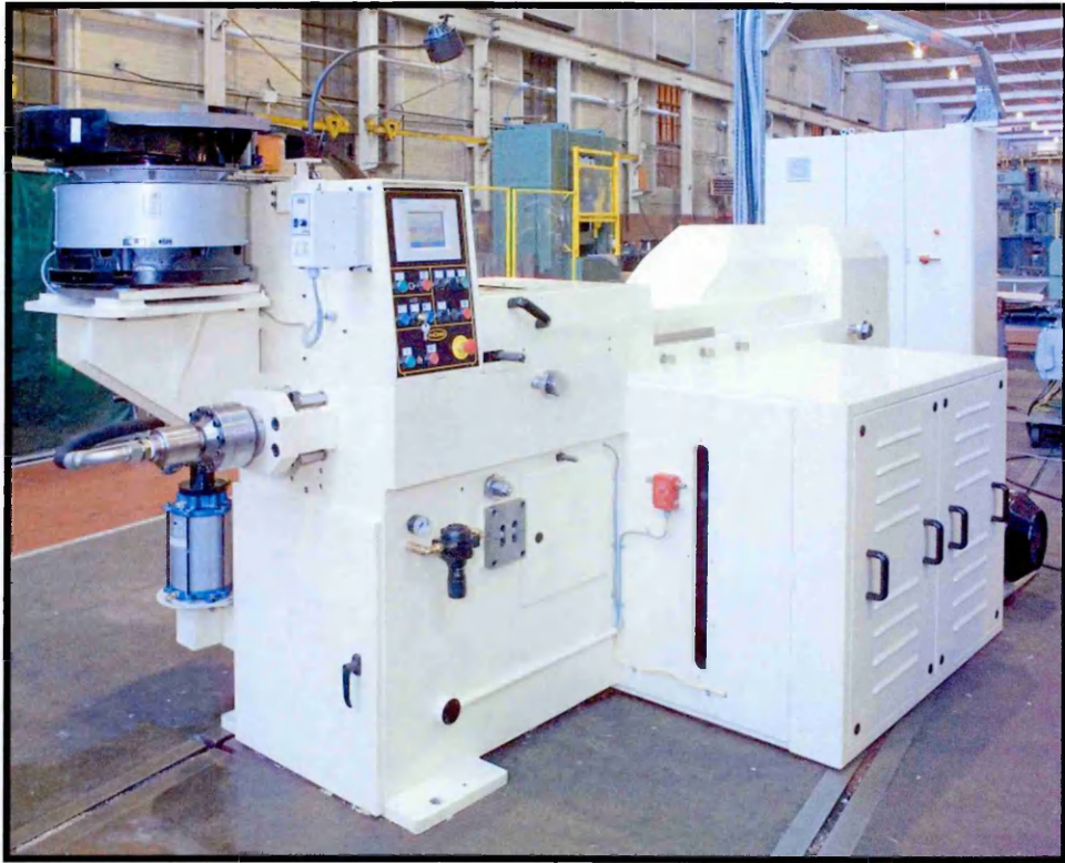
Figure 52: View 1 - Typical Joseph Rhodes Knuckle Joint Press
